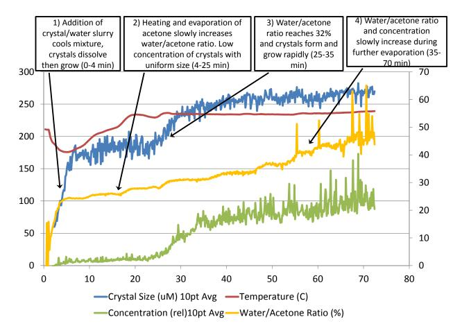
This experiment demonstrates that the MCP probe provides key measurements of crystallization processes. Monitoring these key parameters can lead to a better understanding of the process, as well as better control of final particle size and concentration.
